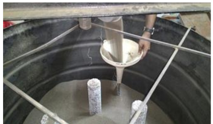
Fig. 8: Filling of sand inside the tank containing pervious concrete piles
