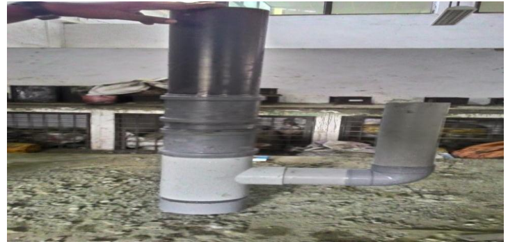
Fig. 2: Falling head permeability apparatus
