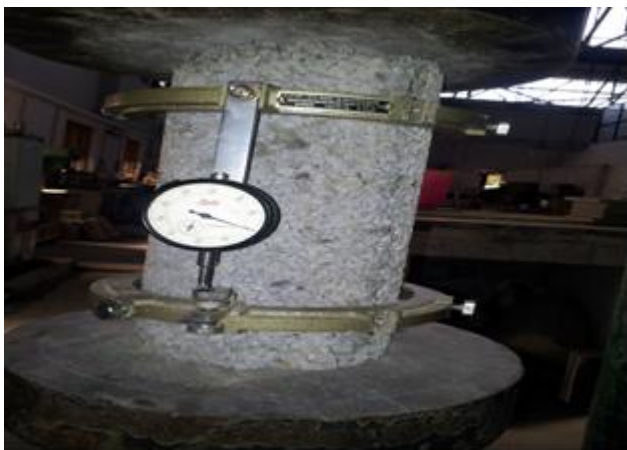
Fig. 6: Setup to find out Modulus Of Elasticity
