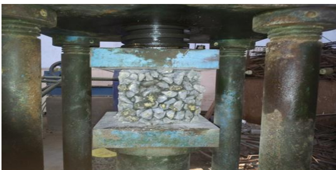
Fig. 1: 16 mm aggregate cube
