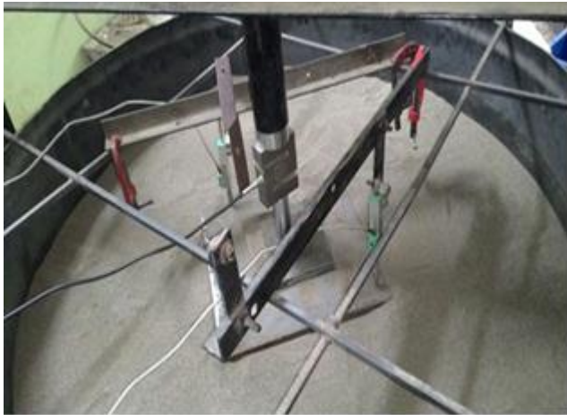
Fig. 9: Test set up for testing group pile
